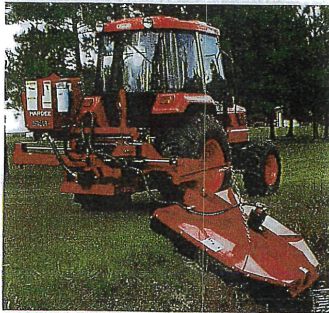
DB4045 48" Hydraulic Drive, Offset Rotary Cutter Complete *
